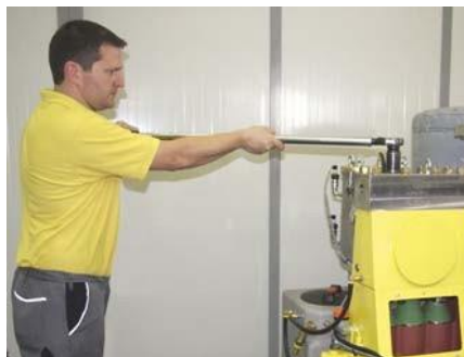
Step 2: Remove the pump head nuts
